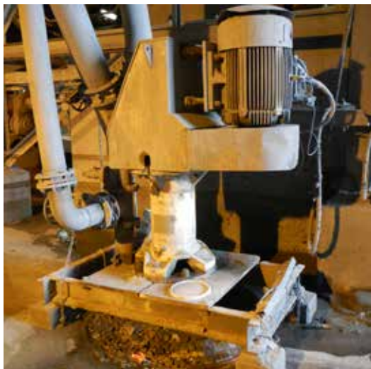
Left and below: The Warman® SPR pump in operation in differing sump environments.
