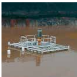
Top Right: SPR pump operating in coal sump application.
