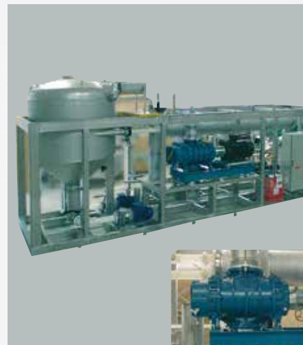
• Engineering: treatment of oil emulsions and cleaning liquids by means of thermocompression concentration system. Lobe blowers (RBS)
