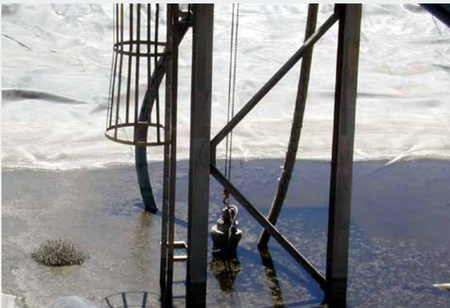
Warman® SHW submersible pump in service at a gold mine.
