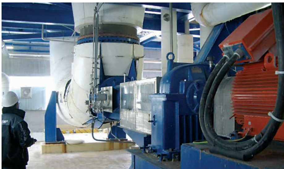
Austria Salt, pump type QCL 1300, Alloy 31/Monel 400
